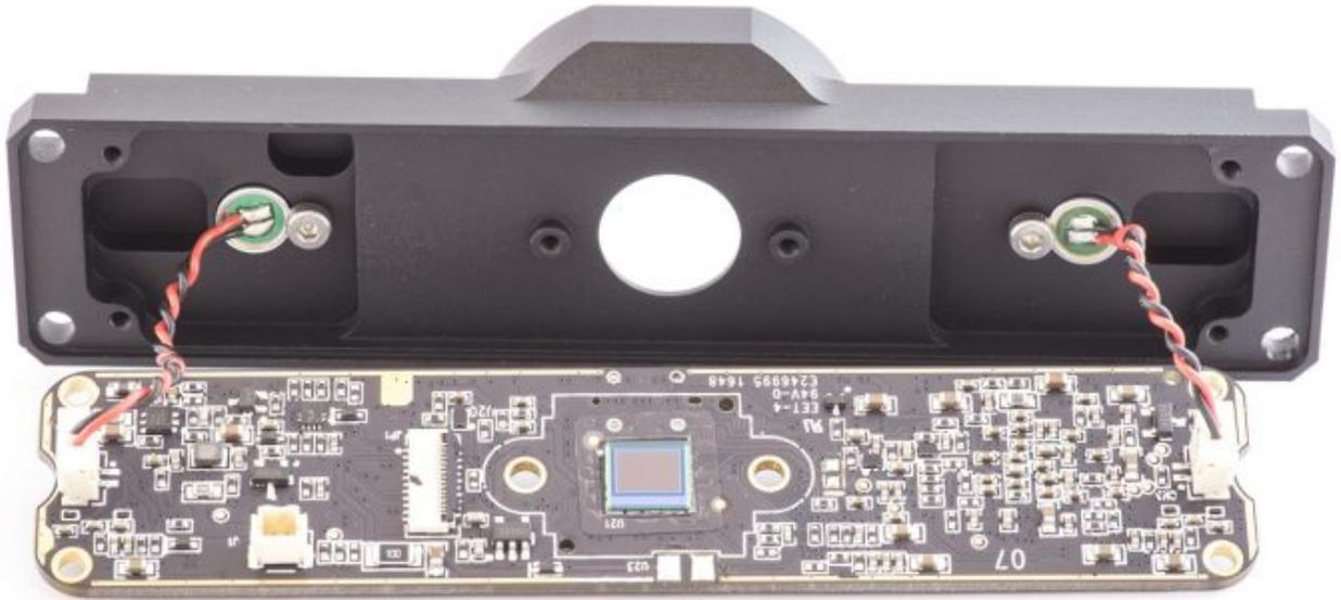
Use included hex key to screw six DIN912 screws. Make sure microphone cables are not pressing against camera board or components. Use tweezers to manipulate them.
