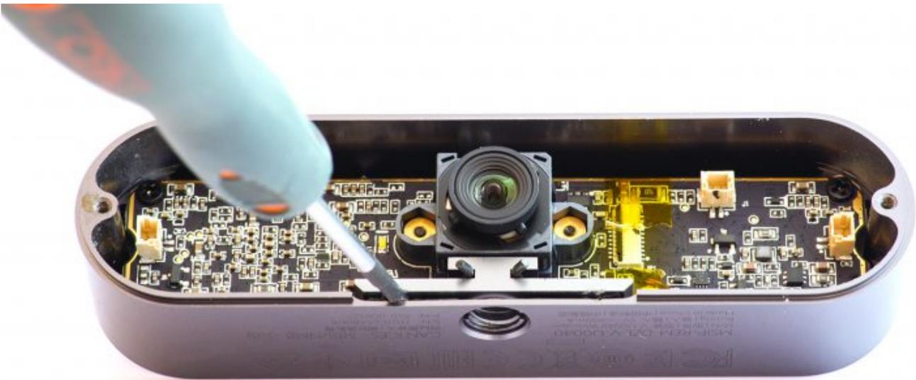
Camera PCB is held by four Philips screws. Undo them to separate board from enclosure.
