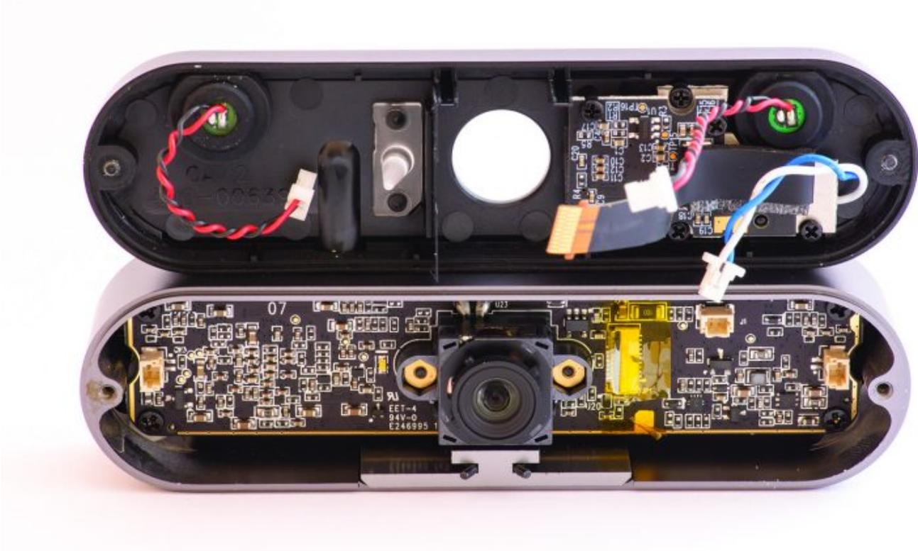
Mount plate is attached to enclosure with double sided adhesive tape. Pry small screwdriver or other flat sharp tool to separate them. Wiggle to remove and be gentle not to damage PCB.
