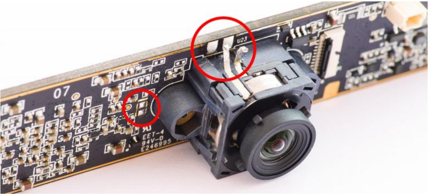
Lens assembly is held together by two screws. This is last tear-down operation. Be careful not to leave your fingerprints on the sensor. If you don't feel comfortable with bare sensor exposed to your workbench, leave it attached for now and remove right before screwing camera PCB into new enclosure.
