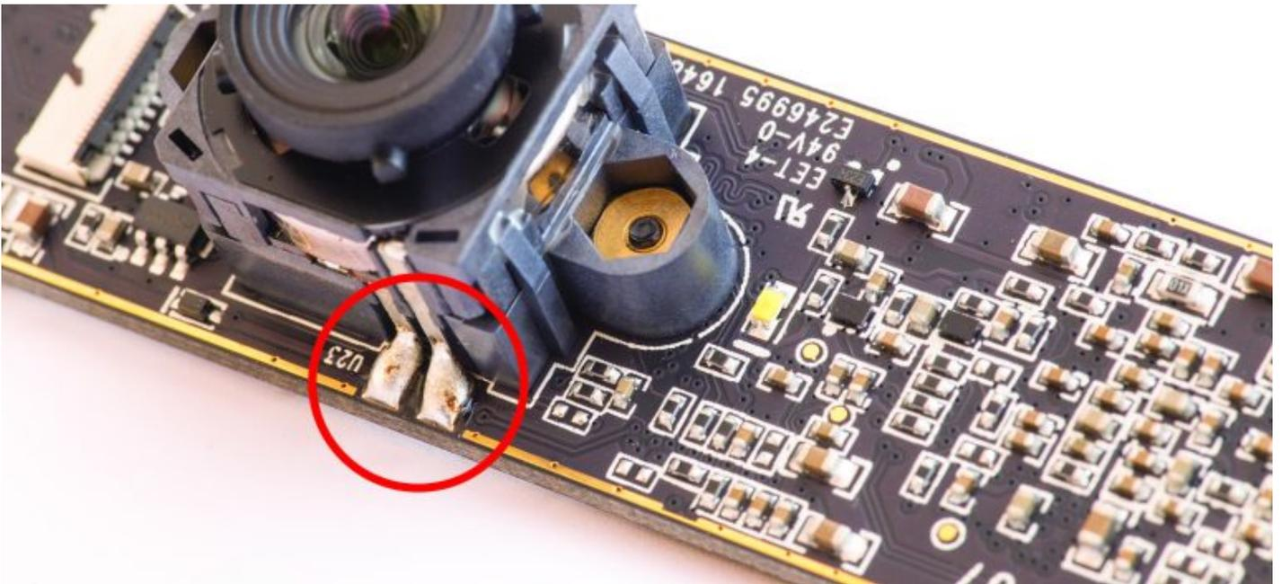
After detaching these components PCB should look like this. It is the only soldering operation required.
