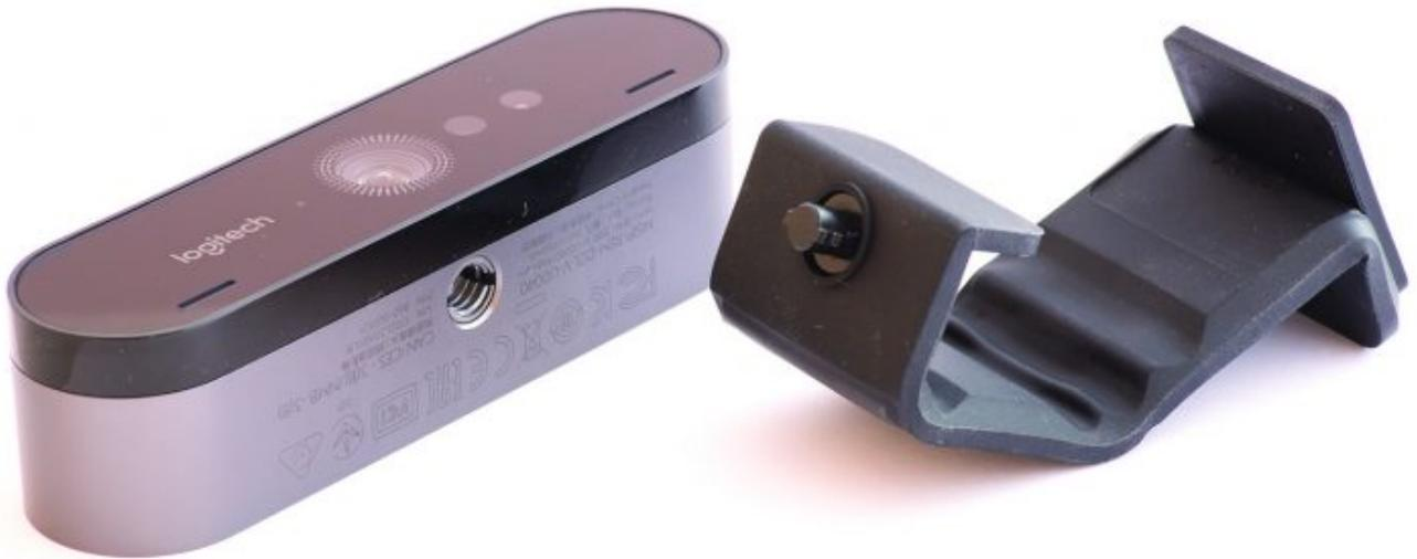
Remove glued plastic front plate. Use small screwdriver, tweezers or other sharp object to pry inside and peel it off.
