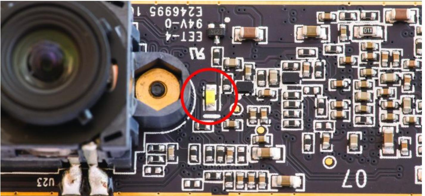
Lens focusing coil is soldered to PCB. These pins also must be un-soldered.
