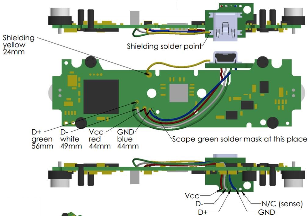
USB connector is available on the other side of PCB and it is surface mount type. Therefore it will be easier to use test pins. While GND is not available as test pin I recommend making pad by yourself. You can also use other places to solder GND wire, it is just my recommendation. Scrape
