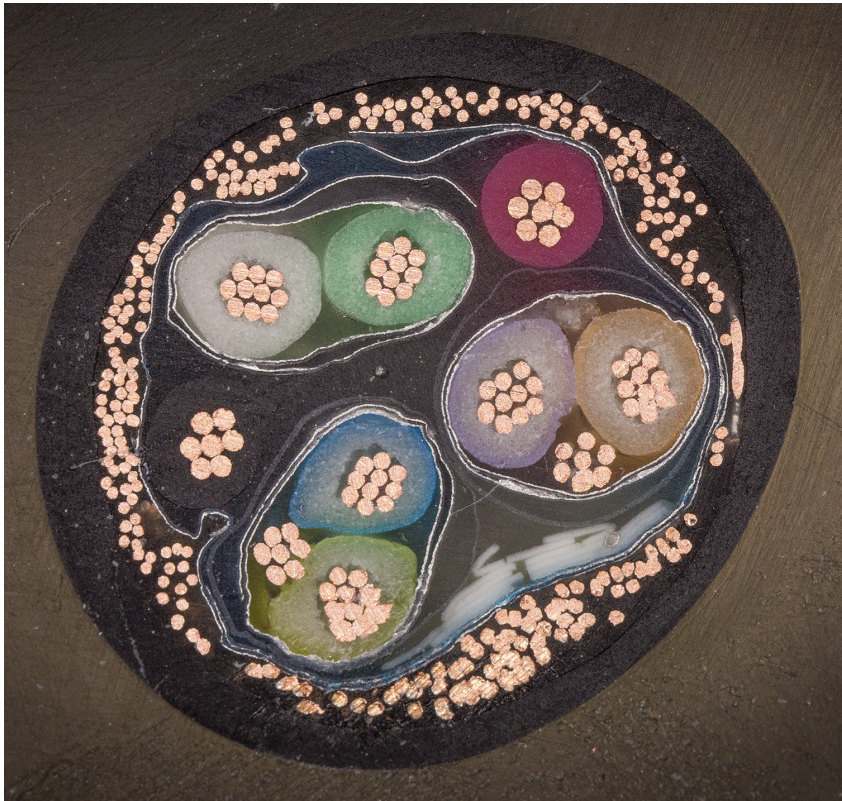
Potted cable cross-section
