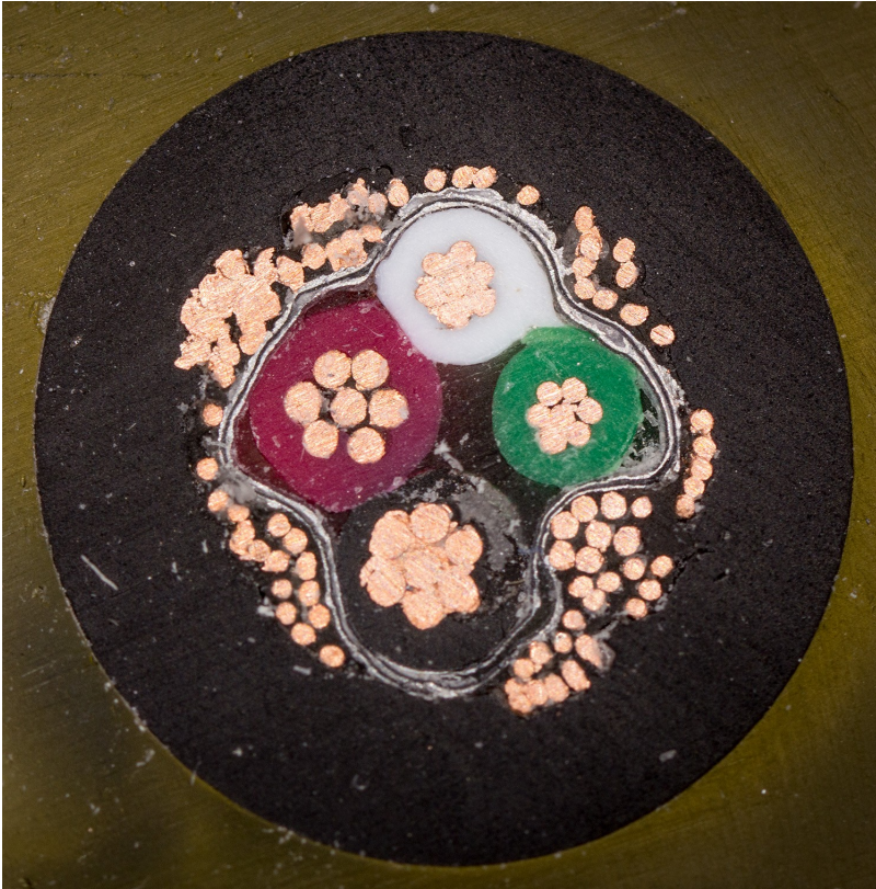
Potted cable cross-section
