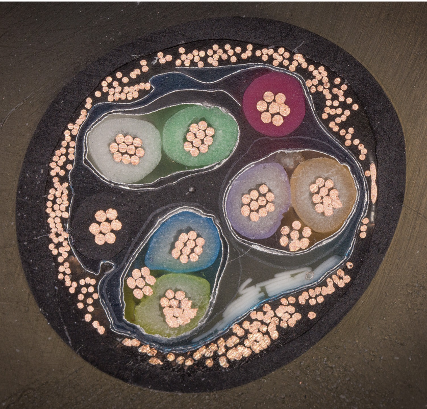
Potted cable cross-section
