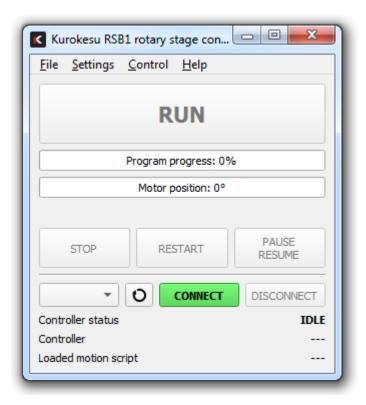
At the same time script processor is very flexible and allows selection from many modes and multiple parameters. Once script/recipe is fine tuned it can be saved for later use.
