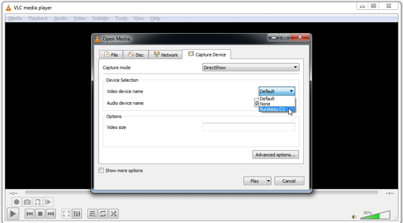
There is one more nifty parameter hidden under `Show more options` checkbox. By default VLC uses 300ms to delay camera view. If real-time video is needed, change to 0ms. But disabling cache has bugs and some video sources will not work at all. For initial testing leave caching untouched.
